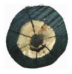
All machining, cutting or drilling of preservative treated timber should be done prior to preservative impregnation. Areas exposed after impregnation due to cross cutting etc., must be treated by liberally applying a suitable paint-on or brush-on remedial or supplemental preservative (excluding ground contact).
